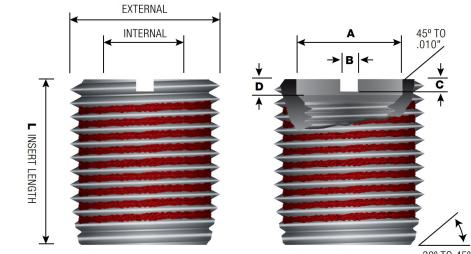
30° TO 45° CHAMFER TO .010" BELOW MINOR THREAD DIAMETER 2X
