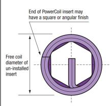
**INSERT SPECIFICATIONS** E Fitted Minor Diameter
